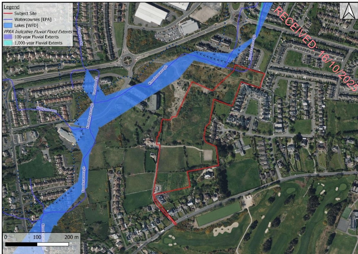
Figure 3-33: PFRA Fluvial Flood Extents
