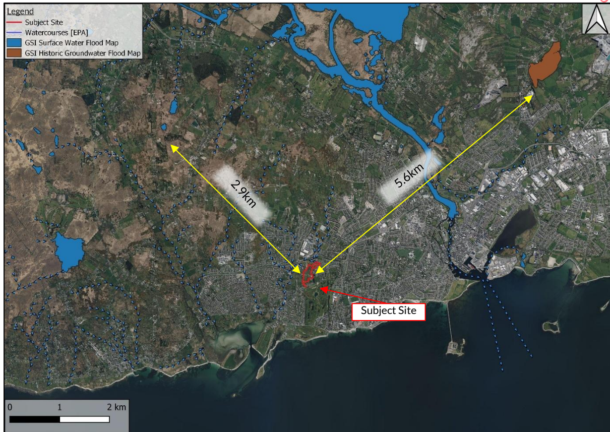
Figure 3-66: GSI Mapping of Groundwater Flooding
